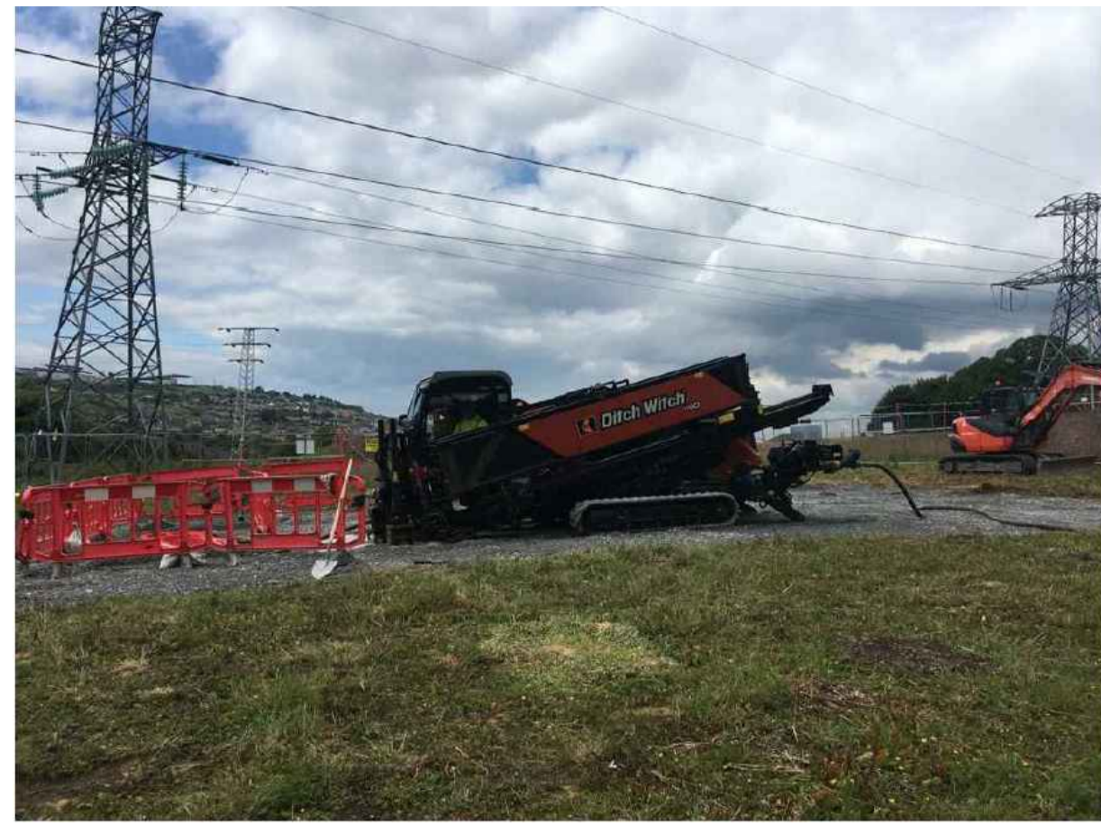
Image 1 : Standard Directional Drilling Rig
