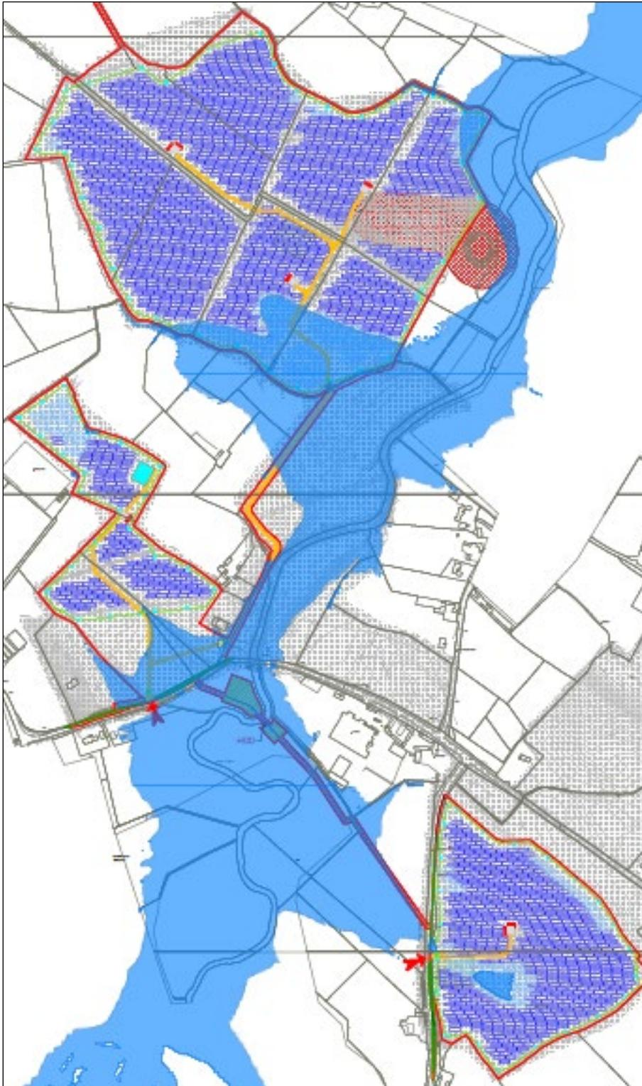
Figure 6-1 Proposed layout and 1% AEP river floodplain (2080)
