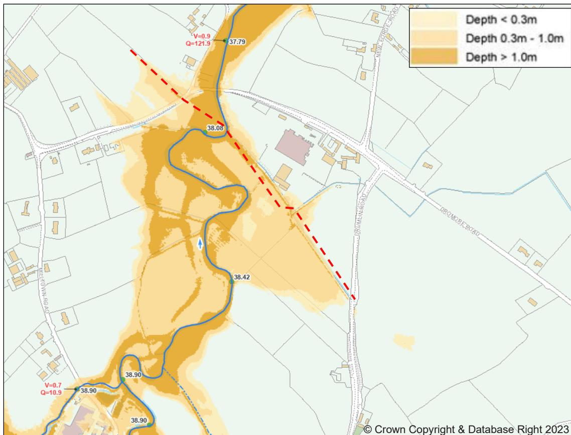
**Figure 6-3 Approximate location of interconnection cable and flood extent (1% AEP, Present day)**
